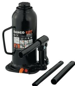
**BAHCO CYLINDER JACK LOAD-BEARING CAPACITY 12 T LIFT 465 MM SCREW-MOUNTED CYLINDER JACK 130 X 150 X 260 MM**
