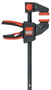
1,00 ST Single-handed clamp EZ clamping width 600 mm radius 90 mm spreading width 195-790 mm
