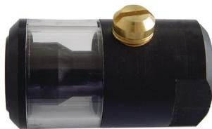
Add-on oil-mist lubricator standard thread mm 11.89 G 1/4 inch flow 750 l/min
