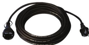
Extension lead with earthing contact 16 A 250 V 3 x 1.5 mm<sup>2</sup> 10 m H05RR-F black
