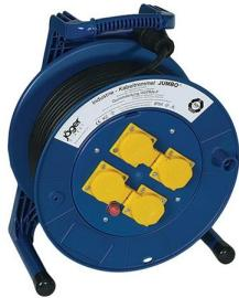
Cable reel 50 m H05RR-F 3 x 1.5 mm<sup>2</sup> 4 sockets with earthing contact solid plastic IP54
