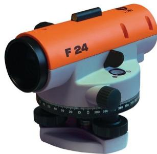
Levelling device F24 object lens diameter 30 mm
