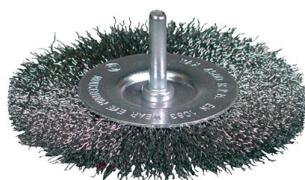
Round brush dm 75 mm wire thickness 0.3 mm VA 10 mm 4500 min<sup>-1</sup>
