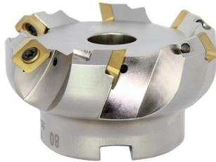
Facing cutter nominal diameter 63 mm nickel-plated with inner cooling no. of cutters 5 SE.. 1204 AF
