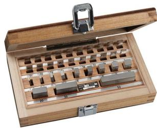
Gauge block set tolerance class 1 32-part steel
