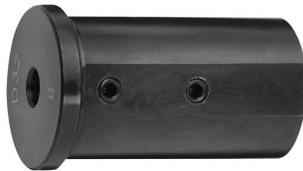
Reducing bushing shape 1 bore dm 12 mm external dm 40 mm clamping length 71 mm L.71mm dm40mm
