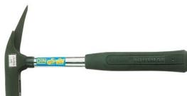
Roofing hammer DIN 7239 head weight 600 g w/o magnet roughened steel pipe, painted black
