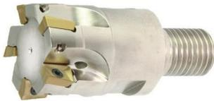
Screw-type mill diameter 25 mm nickel-plated with inner cooling no. of cutters 4 APKT...-10
