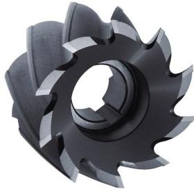
Shell end mill DIN 1880 type N nominal diameter 40 mm HSS-Co5 TiCN no. of cutters 8
