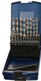
Twist drill set DIN 338 type VA nominal diameter 1-10.5 x 0.5 mm HSS-Co 24-part plastic box
