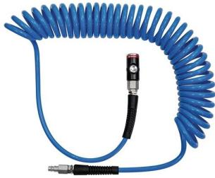
Spiral hose set internal dm 8 mm external dm 12 mm length 6 m safety coupling DN 7.4
