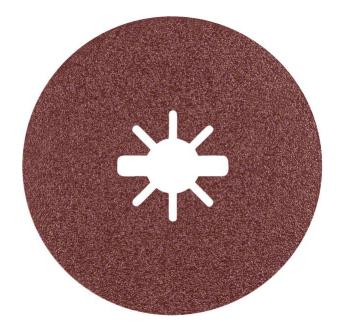
ROBERT BOSCH POWER TOOLS GMBH EXPERT R781 PRISMA CERAMIC X-LOCK FIBRE DISC 115 MM, 22.23 MM, G 60, 5-PC. FOR SMALL ANGLE GRINDERS
