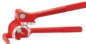
1,00 ST Pipe bending pliers Minibend length 270 mm for pipe diameter 6-8-10 mm bending radius 180 deg
