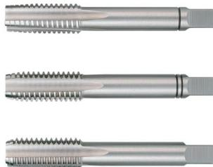
**RUKO SET OF HAND TAPS DIN 352 3-PART M 14X PITCH 2 MM HSS BRIGHT, STRAIGHT, GROOVED ROUGHING/SECOND/BOTTOM. TAP TOL. ISO26H**
