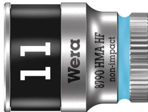
Socket bit 8790 HMA HF 1/4 inch hexagon spanner width 11 mm length 23 mm
